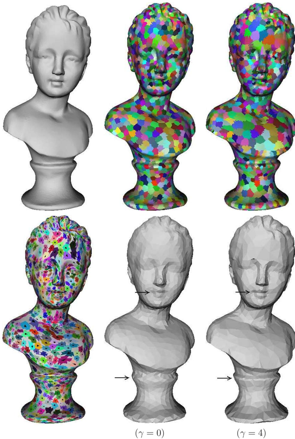
Figure 3.10: A comparison between uniform and adaptive coarsening. Top left: The original Bust model consists of 30.6K vertices. Bottom left: Initialization with  $l$ -neighborhood for level  $l = 3$  resulting in  $k = 2272$  clusters. Top: clustering result and bottom: corresponding triangulation, for different values of  $\gamma$ , respectively.
