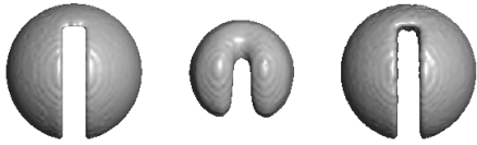
Figure 6: 360° rotation of Zalesak's sphere (100 advect-ions): initial, LS, and PLS. 524,288 particles, 128 3 grid, 14.74 FPS.
