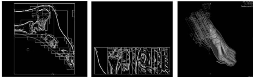
Figure 48.7: Gradient sub-textures defined by the boxes enclose all the voxels of non-zero gradient magnitude (left). The gradient sub-textures are packed into a single larger texture (middle). Resulting rendering of the foot with mixed boxes and textures.
