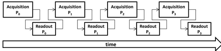
Fig. 1: Schematic view of the acquisition process of a PMD frame using four phase images.
