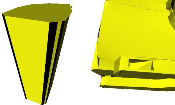
**Figure 6:** Applying polygon reduction only. Left: The upperdeck with holes. Right: A close-up to the arm-rest of the seat with holes and cracks. Both models have been reduced by 90%.
