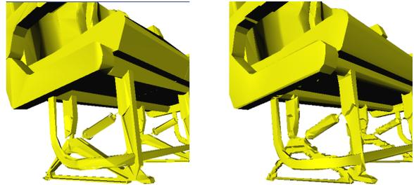
**Figure 8:** The seat base. Left: Only QSlim was applied; the model exhibits several large holes. Right: Model repair and polygon reduction were both applied. The models have been reduced by 90%.
