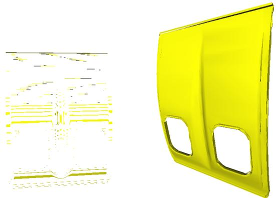
**Figure 9:** The side plate. Left: Attempt to repair the very thin model. Right: Reconstructing an iso-surface for  $d_G \approx 1\%$  of object's size. Both models have been reduced by 90%.
