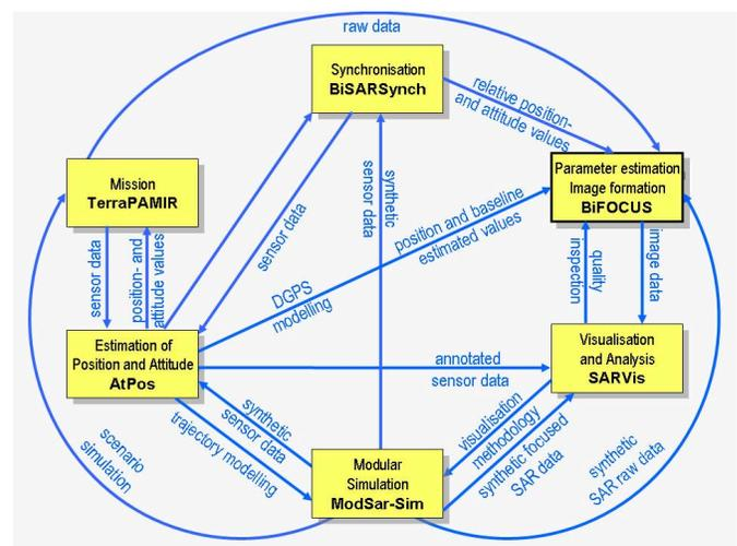
Fig. 1. Interplay between the six topics of the 'bistatic exploration' project.
