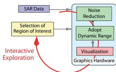
Fig. 6. Conceptual SAR data processing on the GPU
