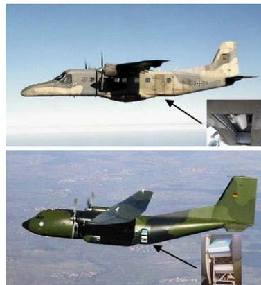
Fig. 3. Bistatic airborne/airborne SAR experiment with PAMIR and its precursor AER-II.
