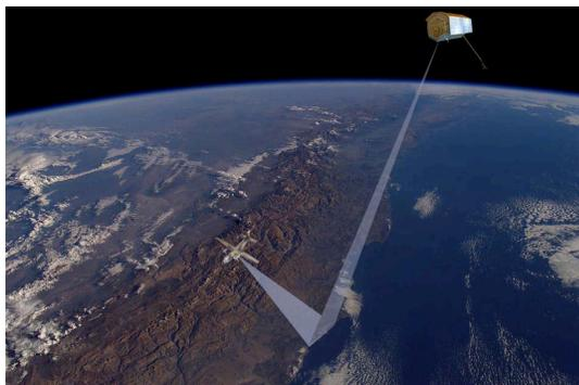
Fig. 2. Artist impression of the planned hybrid bistatic spaceborne/airborne SAR experiments between TerraSAR-X and PAMIR.
