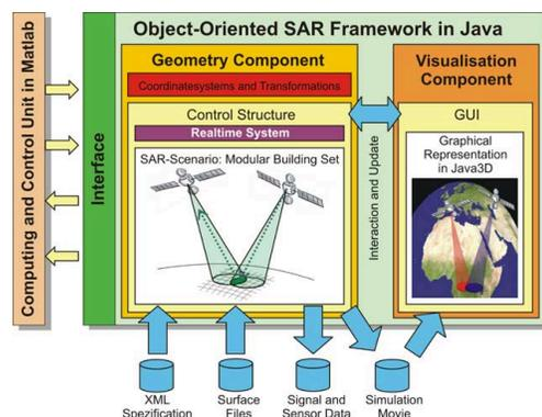
Fig. 5. Architecture of the modular SAR-framework
