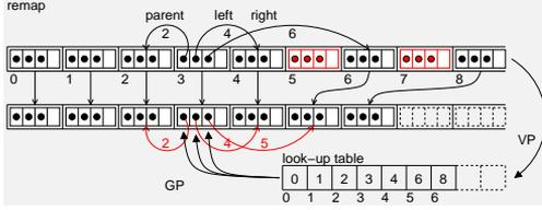
Figure 6: The remap operation. Two nodes (marked red) are removed.
