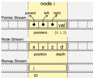
Figure 4: Representation of the tree structure in streams. The cells belonging to one node are marked yellow.
