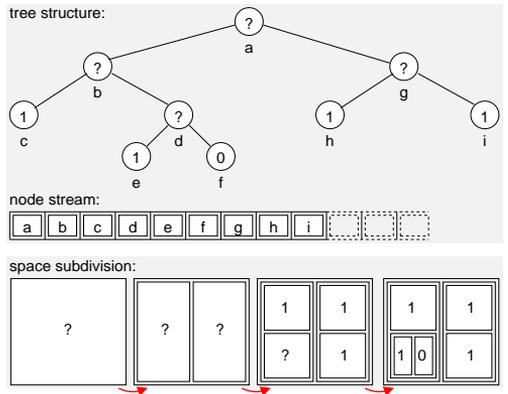
Figure 2: An example (in 2D) consisting of a specific tree and its corresponding spatial representation. The node stream results from a pre-order tree-traversal.
