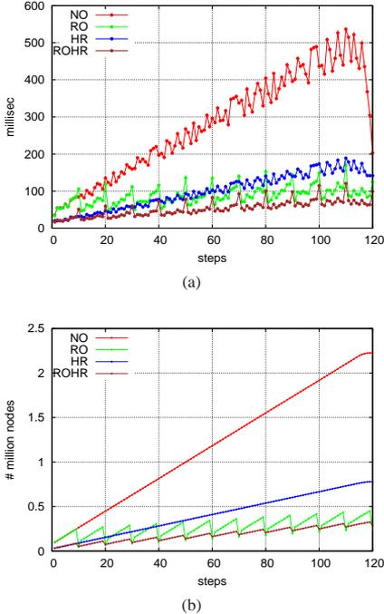
Figure 7: Performance-comparison of different strategies using the write and collapse operations (see Sec. 5.3 for legend’s abbreviations). A torus is drawn in 120 steps (x-axis). In 7(a) the time for writing the new data into the DVT is measured in milliseconds (y-axis). 7(b) displays the total number of nodes (fill-level) during the drawing.
