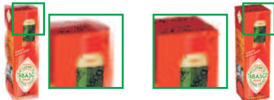
Figure 4 Left: Heavy ghosting artefacts appear without per-pixel depth correction. Right: With depth correction ghosting artefacts can be reduced to a minimum.
